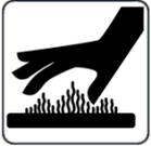
**Hot PARTS HAZARD** All welded pieces become extremely hot immediately after welding or cutting, causing burns to anybody in touch with exposed skin. After welding or cutting, do not contact the workpiece, ground clamp, or electrode holder/torch instantly, and wait for a cooling interval before picking them up. To avoid burns, use proper equipment while working with hot parts, and use thick insulating welding/cutting gloves and clothes as well.
