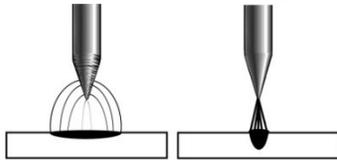
Use only diamond wheels for cutting and grinding. While tungsten is a highly hard material, a diamond wheel's surface is even harder, which allows for more precise grinding. Weld inconsistency and weld flaws can be caused by grinding with aluminum oxide or other non-diamond wheels because they can produce jagged edges, irregularities, or poor surface finishes that are not visible to the naked eye.
