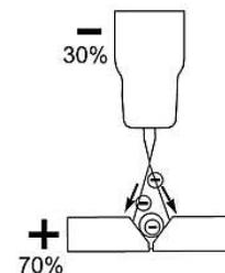
The arc's intensity is proportional to the current flowing from the tungsten. To control the power of the arc, the welder alters the welding current. Thin material typically requires a less strong arc with less heat to melt the material, requiring less current
