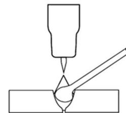
This method is recommended for welding from one side with plate thicknesses more than 6 mm.
