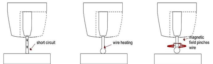
A short circuit results from the wire touching the workpiece. There is no arc because there is no gap between the wire and the base metal.
