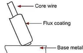
By quickly contacting the electrode to the base metal, the arc is started. At the electrode's end, a molten pool is created as the heat from the arc melts the base metal's surface. The molten pool is where the melted electrode metal is moved across the arc to create the deposited weld metal. A slag that results from the electrode coating covers and shields the deposit. There is a protective gas surrounding the arc and the surrounding areas.
