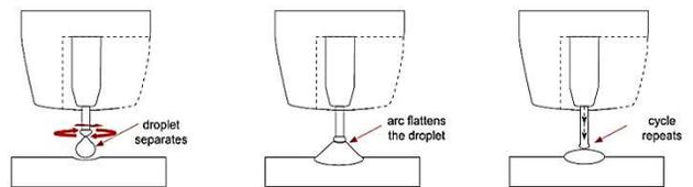
The pinch separates the droplet as it forms, and it then falls into the weld pool that is currently developing.
